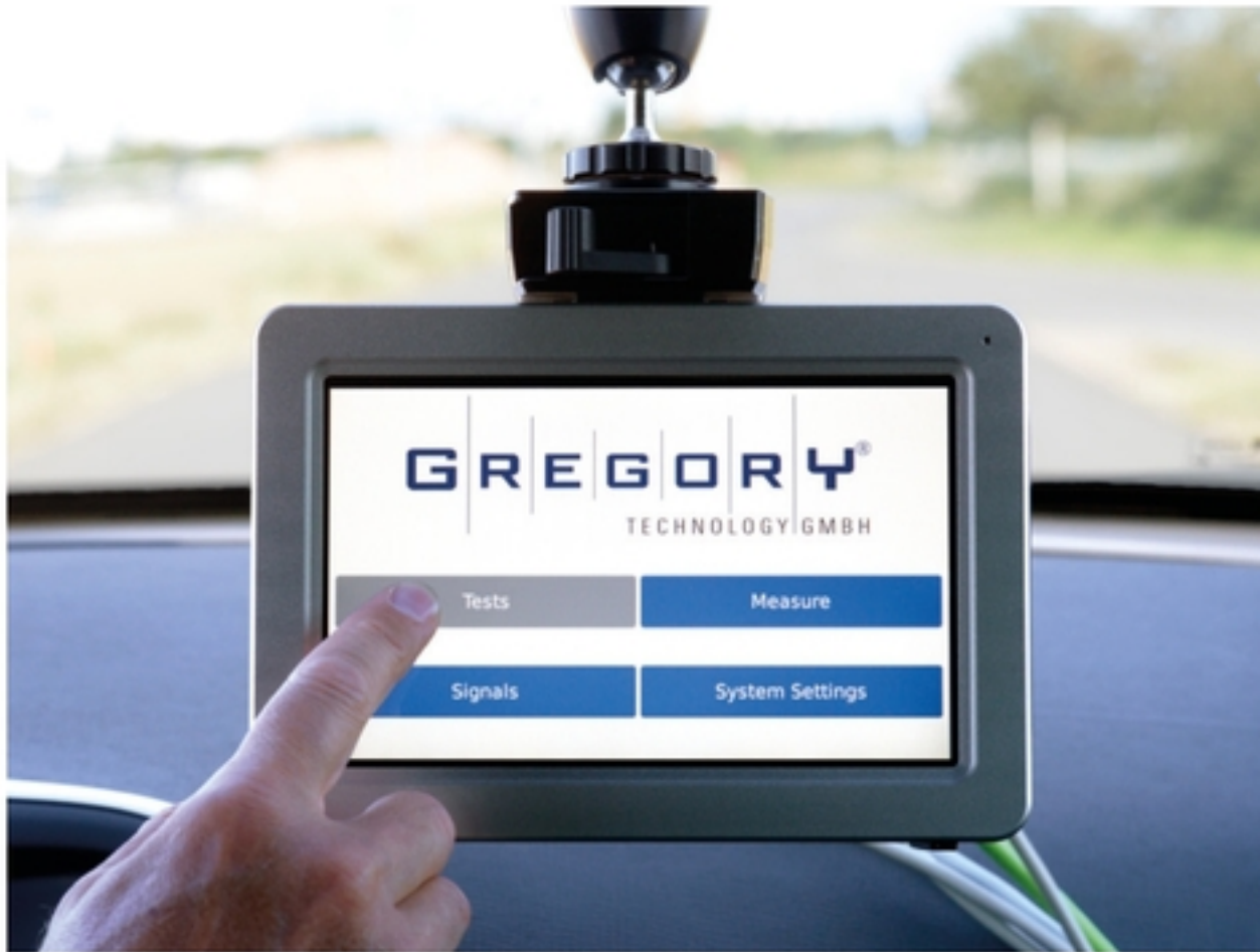
The system has an extra-bright 7in touchscreen color display with easy-to-navigate functions and menus, which guide the user through the entire test analysis process
