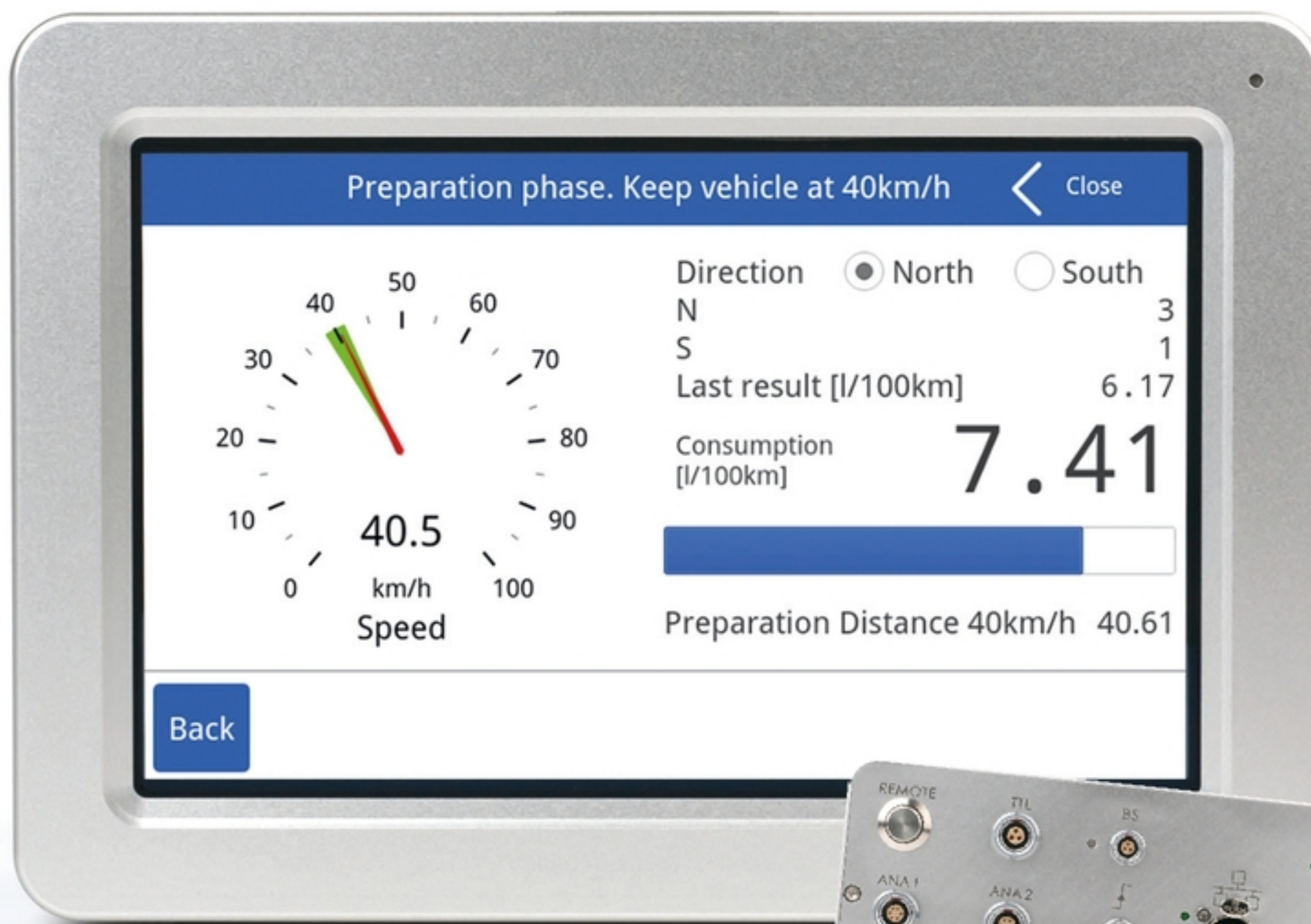
ABOVE: During test runs, the driver benefits from a largely predefined test workflow, which provides maximum support through interactive visual user guidance
